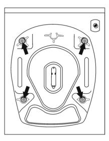
Loosen the bolts by rotating counterclockwise with a suitable spanner.
